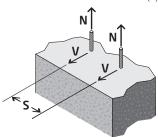
To achieve published tension and shear loads the anchors should be installed at least 12 x the anchor diameter between each other. If spacing between anchors is closer than 12 x the anchor diameter apply appropriate reduction factor as outlined in the SPACING TABLE to the published load to ascertain the reduced load.
