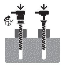
Install with either a socket or cordless impact driver. Apply pressure against the fixing and rotate to engage the first thread. Continue to tighten the anchor until flanged head is firmly seated against fixture.
